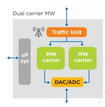
MPU: MW Carrier: E-band Carrier: Traffic Unit: DAC: Handles the radio link configuration & monitoring and some specific PHY layer control loops Includes all the modulation and demodulation functions for the microwave RF carrier Includes all the modulation and demodulation functions for the millimeter wave RF carrier Implements the Ethernet L1 traffic handling
